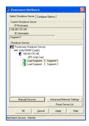
Shut down individual load segments without powering down all connected equipment.
