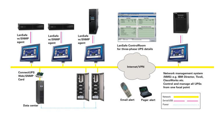
LanSafe provides comprehensive support for both Eaton single-phase and three-phase and Eaton MGE Office Protection Systems single-phase UPS products via serial, USB and network connectivity options.
